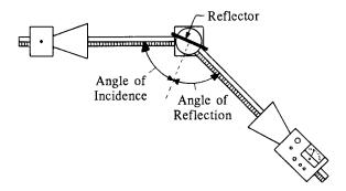
Figure 2: Angles of Incidence and Reflection
