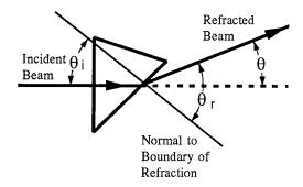
Figure 5: Geometry of Prism Refraction
