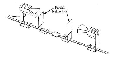
Figure 13: Fabry-Perot Interferometer
