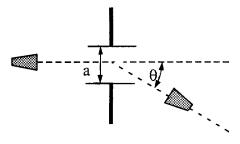
Figure 11: Single-Slit Diffraction
