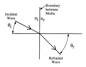
Figure 3: Angles of Incidence and Refraction
