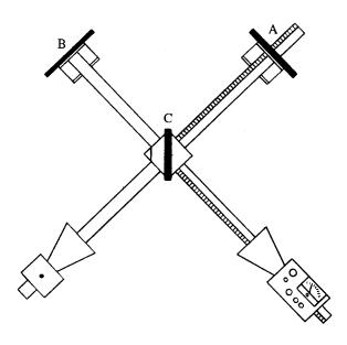
Figure 14: Michelson Interferometer
