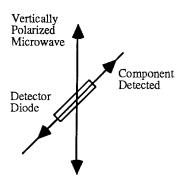
Figure 7: Detecting Polarized Radiation
