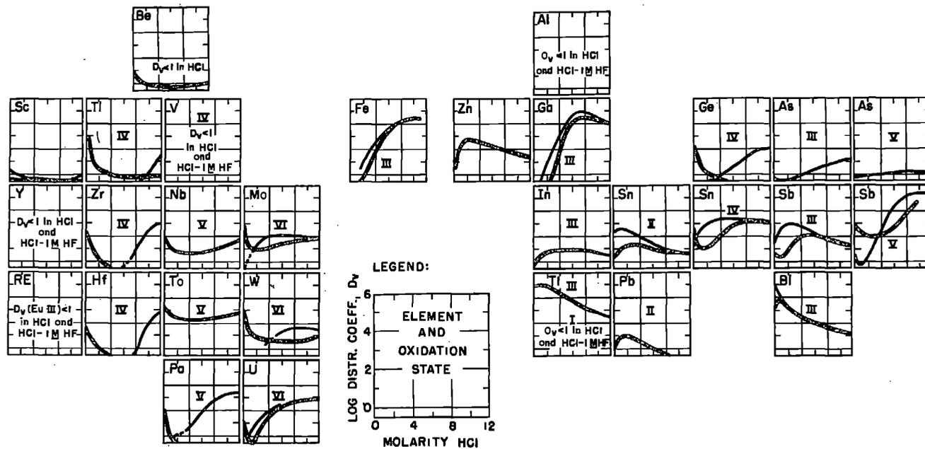
Figure 69. Adsorption of elements from HCl and HCl-HF solutions with anion exchange resin. — Distribution coefficients in absence of HF. - - - - - Distribution coefficients in HCl-HF mixtures (usually 1M HF except Zr(IV), Hf(IV), Nb(V), Ta(V), and Pa(V) where  $\frac{M}{HF} = 0.5$ ). After F. Nelson, R. M. Rush, and K. A. Kraus, reference 558.
