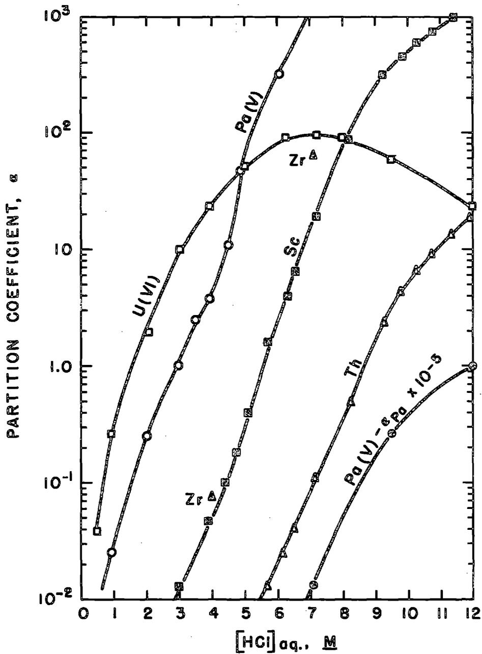
Figure 38. The extraction coefficient of U, Pa, Th, Zr, and Sc between pre-equilibrated 100% TBP and aqueous hydrochloric acid at  $22^{\circ} \pm 2^{\circ}C$ . After D. F. Peppard, G. W. Mason, and M. V. Gergel, reference 429, and D. F. Peppard, G. W. Mason, and J. L. Maier, reference 422.
