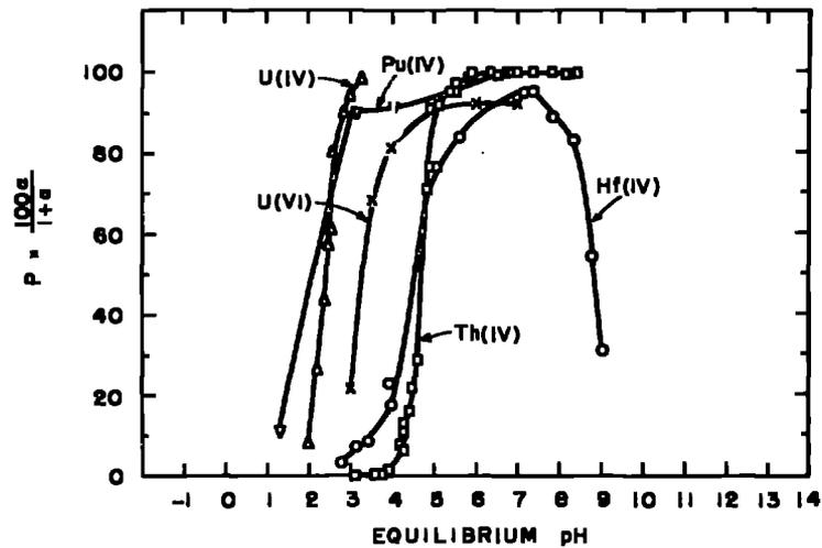
Figure 54-A. The extraction of various elements from 0.1M NaClO<sub>4</sub> solutions by an equal volume of acetylacetone-chloroform solution at 25°C. Acetylacetone concentrations used: U(VI), 0.0210M [HAA]<sub>aq</sub>; U(IV), 0.50M [HAA]<sup>0</sup><sub>org</sub>; Pu(IV), 1.00M [HAA]<sub>init</sub>; Th(IV), 0.0489M [HAA]<sub>init</sub>; Hf(IV), 0.050M [HAA]<sup>0</sup><sub>org</sub>. After J. Rydberg, references 51, 486-488.
