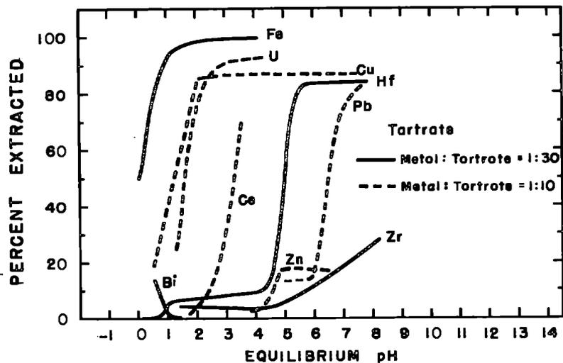
Figure 55-D. The effect of tartrate on the extraction of various metals from aqueous solution by an equal volume of acetylacetone at 25°C. The mole ratio of metal to tartrate is shown by the line texture. After A. Krishen, reference 489.
