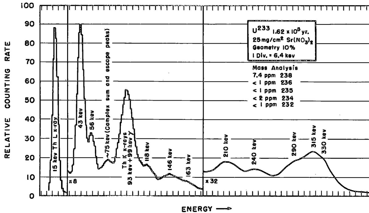
Figure 83. Gamma-ray spectrum of U<sup>233</sup> obtained with a 4-inch diameter x 4-inch thick cylindrical NaI(Tl) crystal. After C. E. Crouthamel, C. Gatrousis, S. J. Gaslovich, reference 649.
