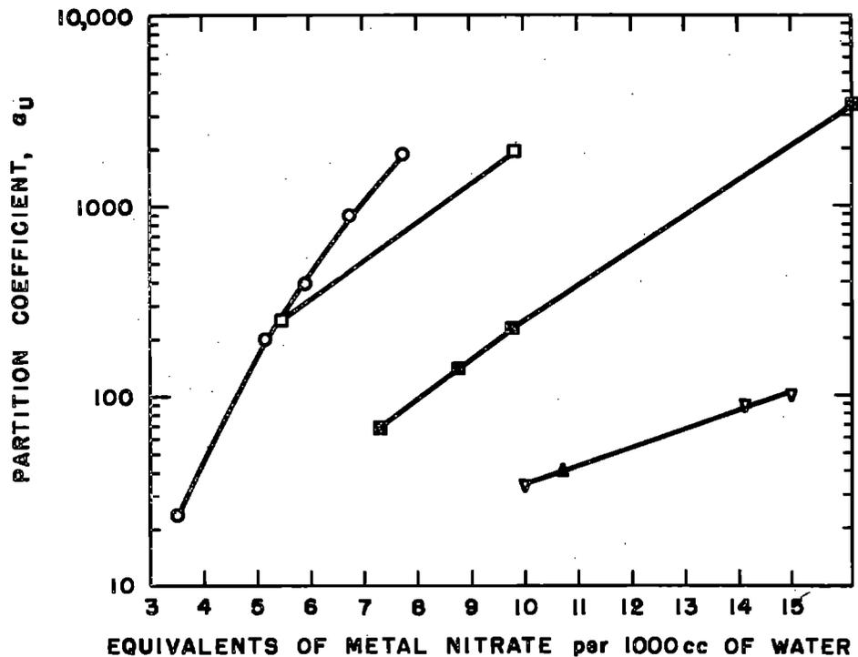
Figure 24. Effect of salting-out agents on the extraction of uranium by pentaether.  $\blacktriangle$   $\text{NaNO}_3$ ,  $\nabla$   $\text{NH}_4\text{NO}_3$ ,  $\blacksquare$   $\text{Ca}(\text{NO}_3)_2$ ,  $\circ$   $\text{Al}(\text{NO}_3)_3$ ,  $\square$   $\text{Fe}(\text{NO}_3)_3$ . After E. Evers and C. Kraus, reference 332. Conditions: Uranium concentration, 2-6 g/100 cc of phase. Temperature, 27°C or room temperature.
