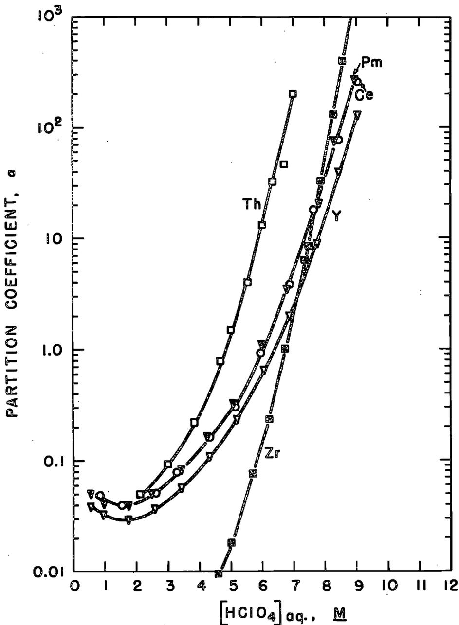
Figure 44. The distribution of Th, Pm, Ce, Zr, and Y between 100% TBP and aqueous solution as a function of initial equilibrium aqueous HClO<sub>4</sub> concentration. After S. Siekierski, reference 433. Conditions: Equal phase volumes (15 ml) shaken together for about 20 minutes at 21°-25°C.
