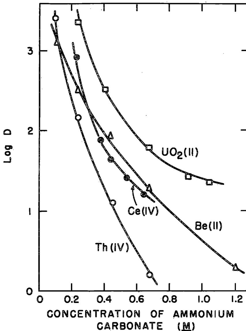
Figure 72. The adsorption of elements from ammonium carbonate solutions with Dowex-1 anion exchange resin (x8, 50-100 mesh). After S. Misumi, T. Taketatsu, reference 575. Conditions: Amounts taken,  $\text{Be}^{2+}$ , 11.7 mg ( $\text{BeO}$ );  $\text{Ce}^{4+}$ , 7.3 mg ( $\text{CeO}_2$ );  $\text{Th}^{4+}$ , 26.9 mg ( $\text{ThO}_2$ ); and  $\text{UO}_2^{2+}$ , 61.0 mg ( $\text{U}_3\text{O}_8$ ). 1 gram of resin and 200 ml of solution in contact 12-20 hours at 20°C.
