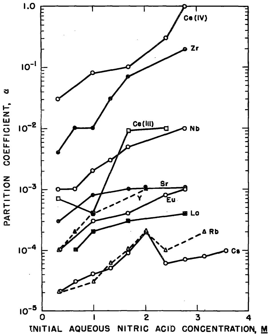
Figure 14. Partition coefficients of fission products between diethyl ether and aqueous solution containing  $\text{Ca}(\text{NO}_3)_2$  and different initial acidities. After V. Vdovenko, reference 344. Conditions: Aqueous solution--required amounts of nitric acid and radioactive material added to 3.5M solution of  $\text{Ca}(\text{NO}_3)_2$ ;  $V_0/V_a$ , 1.
