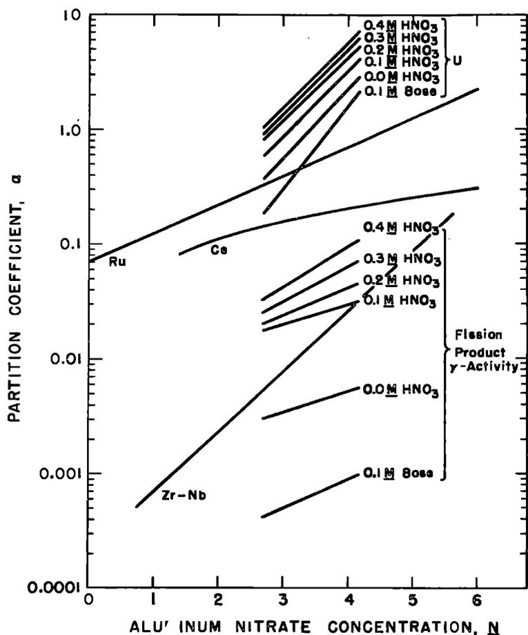
Figure 29. The effect of salting-out agent,  $\text{Al}(\text{NO}_3)_3$ , on the extraction of uranium and fission products by hexone from aqueous solution at various nitric acid concentrations. After F. R. Bruge, reference 378.
