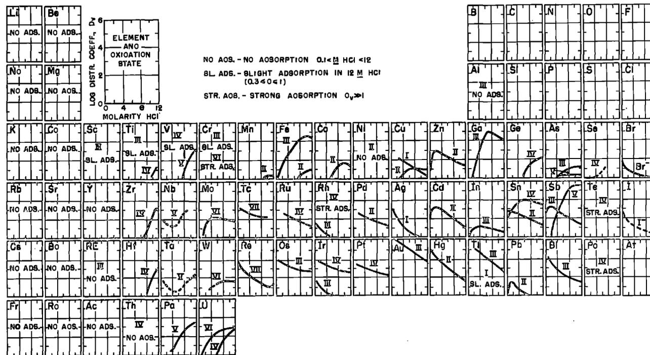
Figure 65. Adsorption of elements from hydrochloric acid solution with anion exchange resin (quaternary amine polystyrene divinyl benzene resin, ~200 mesh, 10% DVB). After K. A. Kraus and F. Nelson, reference 536.
