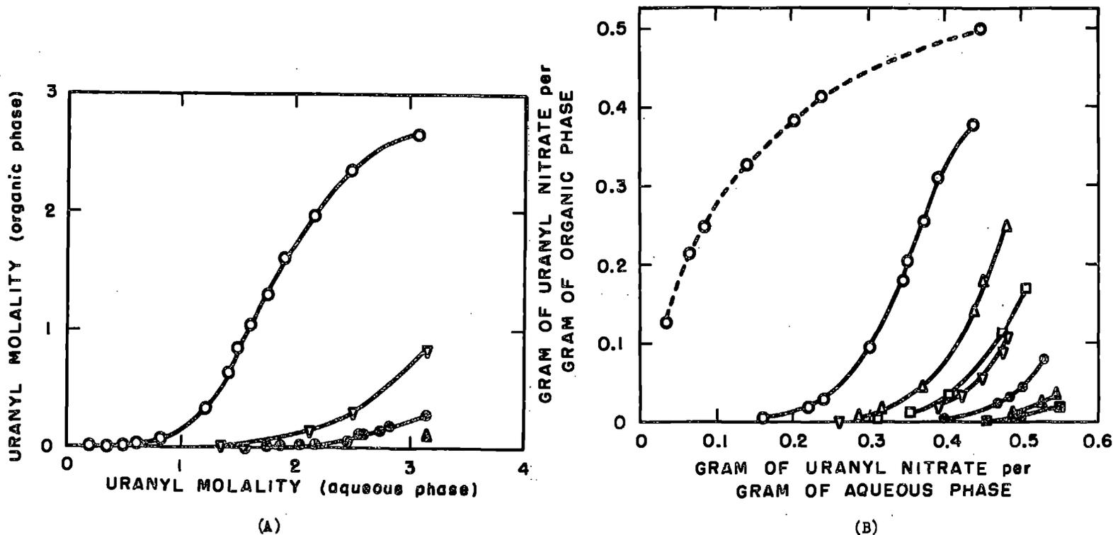
Figure 1. Partition of uranyl nitrate between water and simple ethers. O, diethyl ether. Δ, ethyl-n-propyl ether. □, ethyl-n-butyl ether. ∇, di-isopropyl ether. ⊙, di-n-butyl ether. △, di-n-hexyl ether. □, 2,2'-dichlorethyl ether.
