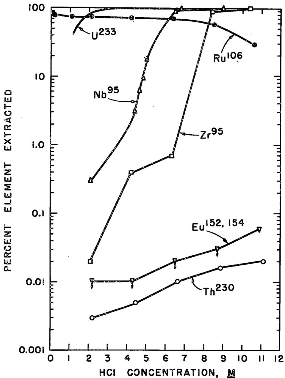
Figure 53. The extraction of U<sup>233</sup>, Th<sup>230</sup>, and fission products by 5% (w/v) triisooctylamine in xylene as a function of HCl concentration. After F. L. Moore, reference 475. Conditions: Equal phase volumes extracted for two minutes at room temperature (24°C.).
