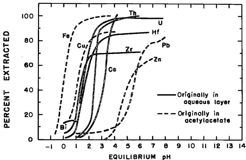
Figure 55-A. The extraction of various metals from aqueous solution by an equal volume of acetylacetone at 25°C. Solid lines indicate the metal was originally contained in the aqueous phase. The dashed lines indicate the metal was originally in the organic phase. The pH was adjusted to the desired value by sulfuric acid or sodium hydroxide. After A. Krishen, reference 489.
