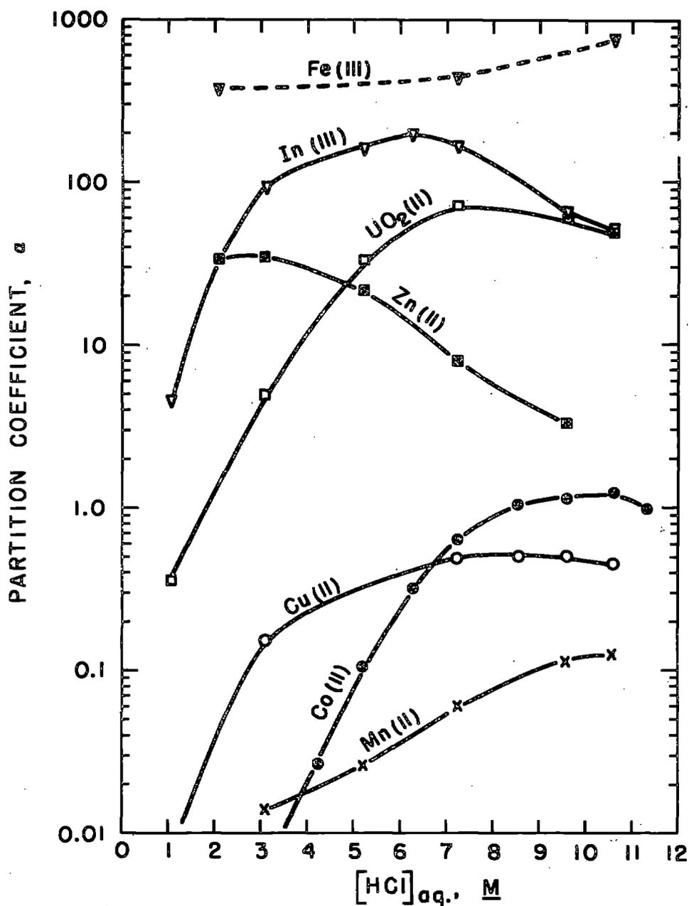
Figure 39. The extraction coefficients of U, In, Zn, Cu, Co, Fe, and Mn between pre-equilibrated 100% TBP and aqueous HCl solution at  $21 \pm 0.1^\circ\text{C}$ . After H. Irving and D. N. Edgington, reference 430. Conditions: TBP and HCl pre-equilibrated by stirring equal volumes together for about 10 minutes. Tracer concentrations of about 0.02M U and Cu used. Equal volumes of pre-equilibrated phases stirred together about 5 minutes.
