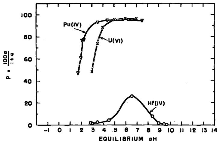
Figure 54-C. The extraction of various elements from 0.1M NaClO<sub>4</sub> solutions by an equal volume of acetylacetone-hexone solution at 25°C. Acetylacetone concentrations used; U(VI), 0.0210M [HAA]<sub>aq</sub>; Pu(IV), 1.00M [HAA]<sub>init</sub>; Hf, 0.050M [HAA]<sub>org</sub>. After J. Rydberg, references 51, 487, 488.
