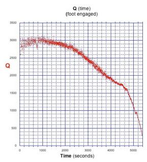
One may now see all three dissipations. I estimate the going amplitude at approximately 30 flag widths or ~ 800 s in the graph on the left. I haven't concluded whether the friction in the rest of the clock affects the Q. However, the system  $Q^6$  of weight driven clocks are easily found. I intend to discuss this, *inter alia*, in part three.
