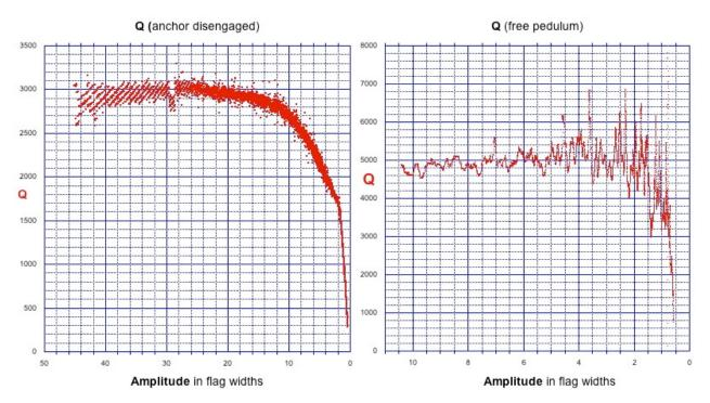
split foot. To the right is shown the last ~ ten flag widths of the same pendulum freely decaying with the expected greater Q. Determination of the dissipation type requires the Q found as a function of the time. So next is the foot engaged Q plotted as a function of the time.
