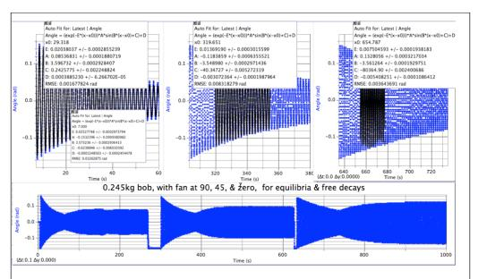
For viscous (linear) dissipation,  $Q \simeq \omega_1 / 2(k/m)$  or  $\omega_1 m / 2k$
