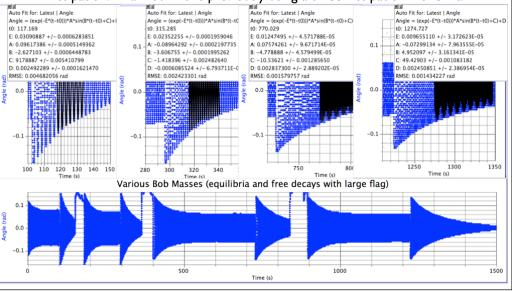
I've shown experimentally, contrary to many's intuition, that the mass of a pendulum's bob does not significantly affect it's driven equilibrium amplitude. However, I had verified in other trials that, characteristically, a driven pendulum responds both in resonance and transient behaviour to its Q, whether the Q value is either due to dissipation and or its bob mass.
