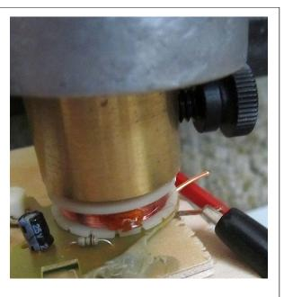
Drive for a faux pendulum from a quartz clock
